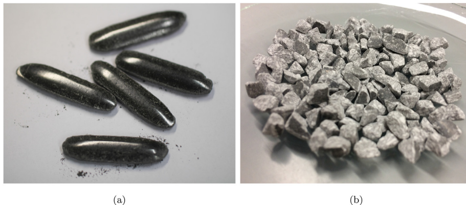
Fig. 3. a): compacted bars of the 97% K_2CO_3 base material and binder. b): bars granulated into final composite granules.
