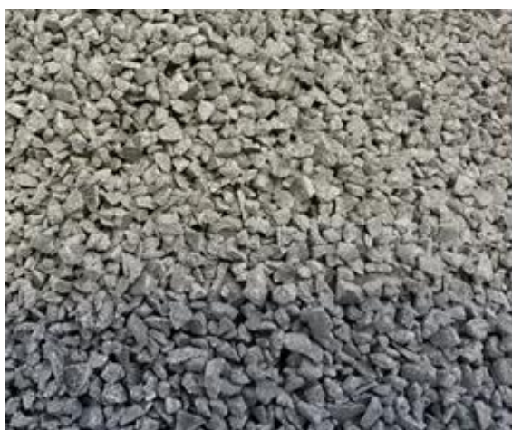
Figure 2: Granules of potassium carbonate ( K_2CO_3 ) that were produced for the CREATE system.
