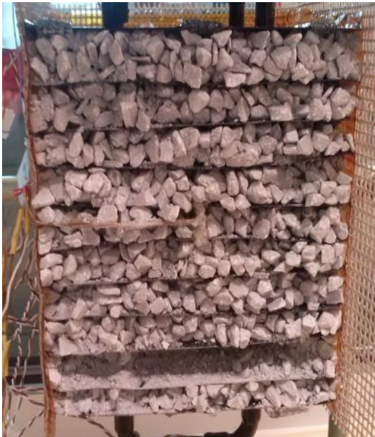
Figure 7: The filled 1 kg heat exchanger.
