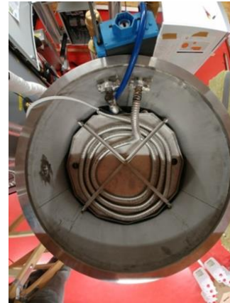
Figure 10: Corrugated tube evaporator/condenser. In the middle the stacking of three dishes can be seen. Right: the evaporator/condenser built into the top part of a stainless steel cylinder. The bottom part of this cylinder is the condensed water storage.
