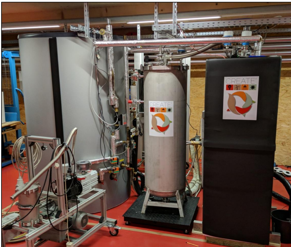
Figure 9: The first prototype absorber module (to the right, packed in insulation material), connected to the evaporator/condenser in the middle and to a hot water tank to the left. The sources and sink were provided by the laboratory infrastructure.
